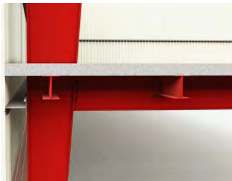
Mezzanine Edge Angle Detail (Longitudinal Direction)
